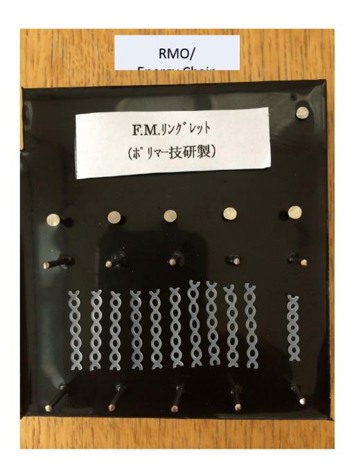
Overall elongation can be observed but the deformation of the rings are not so noticeable and mostly keeping the original shape.
